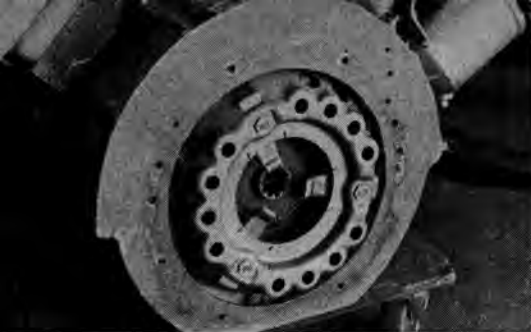
Adaptor plate has been welded in place on Chrysler V8. The clutch used is a Friction-Master and flywheel is from a Chrysler.
